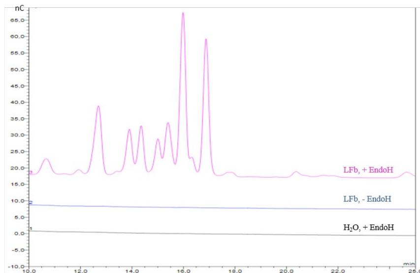
**Column:** Dionex CarboPac PA100,  $\varnothing$ 2 mm. **Eluent:** 100 mM NaOH + 250 mM NaOAc in 100 mM NaOH, 20 °C, 0.3 mL/min. **Injection volume:** 10  $\mu$ L. **Detection:** Disposable gold working electrode, Au-PTFE, coupled with reference electrode Ag/AgCl. **Chromatographic system:** ICS-5000 HPIC, software Chromeleon 6.8.
